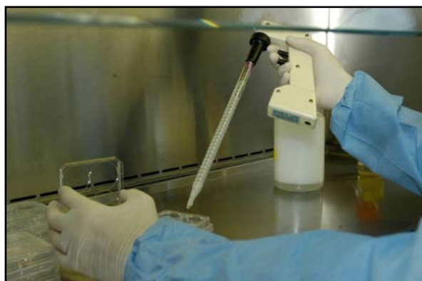
Application of test solution to virus film on coupons in 6-well plate
