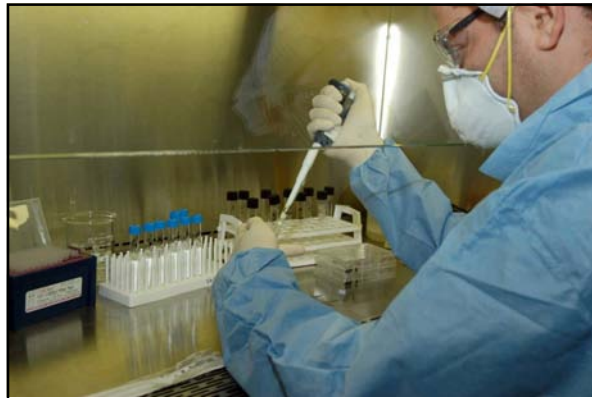
Collected test solution to be diluted, post treatment of virus film on coupon
