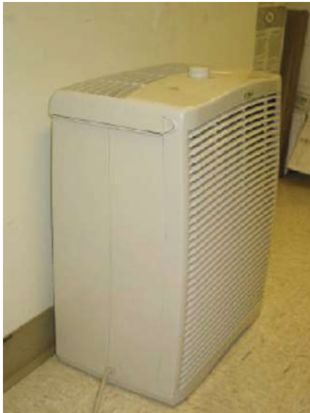
Figure 47. Photograph of In-Room Air Cleaner Used During Testing (Whirlpool Model AP4503H0)
