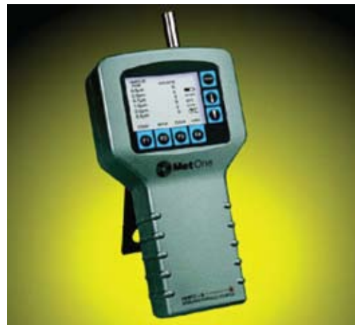
Figure 7. Photograph of MetOne Handheld Optical Particle Counter
