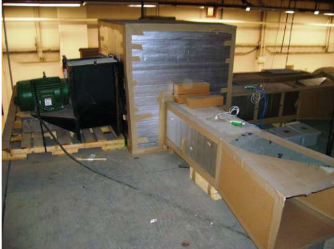
Figure D-7. Photograph of the Downstream Side and Blower of the Test Fixture Used During the Ambient Aging of the Electronic Air Cleaners
