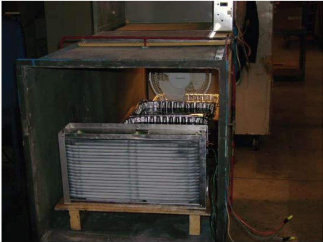
Figure D-6. Photograph (interior) of the Test Fixture Used During the Silicon Vapor Exposures of the Electronic Air Cleaners
