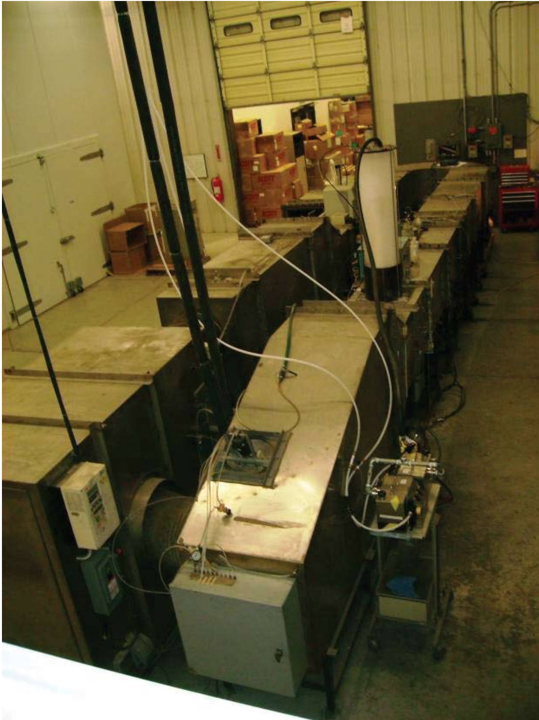
Figure D-1. Photograph of the Upstream Side of Intertek's ASHRAE 52.2-1999 Inert Aerosol Test System Used During the Inert Aerosol Tests and Electrostatic Conditioning Tests
