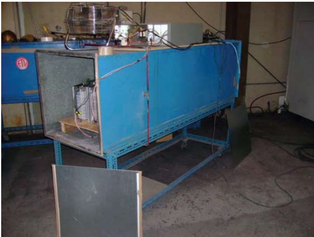
Figure D-5. Photograph (side view) of the Test Fixture Used During the Silicon Vapor Exposures of the Electronic Air Cleaners
