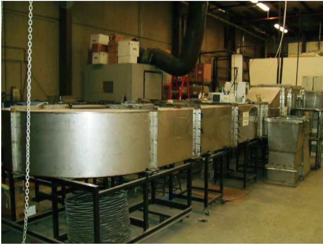
Figure D-2. Photograph of the Downstream Side of Intertek's ASHRAE 52.2-1999 Inert Aerosol Test System Used During the Inert Aerosol Tests and Electrostatic Conditioning Tests
