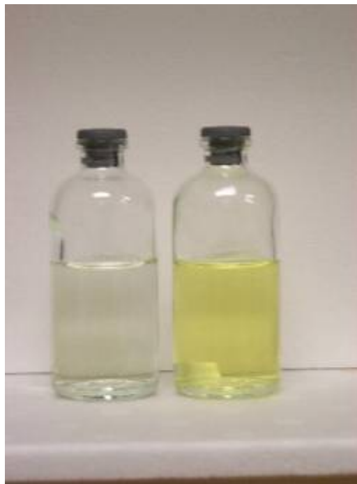
Figure 6. Comparison of OPH-agarose treated (right) and untreated (left) paraoxon in tap water after five days in the 50-ml Pharmed™/glass system. The yellow compound is the p -nitrophenolate ion of p -nitrophenol, one of the paraoxon hydrolysis products.
