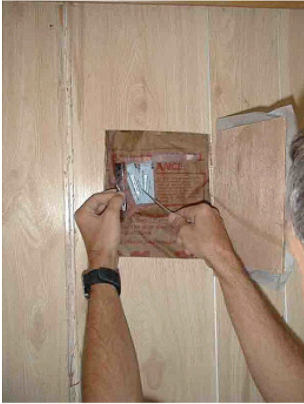
Figure 5.4-5. Spore strip site 3. Left: strips inside wall insulation. Right: paneling in place.
