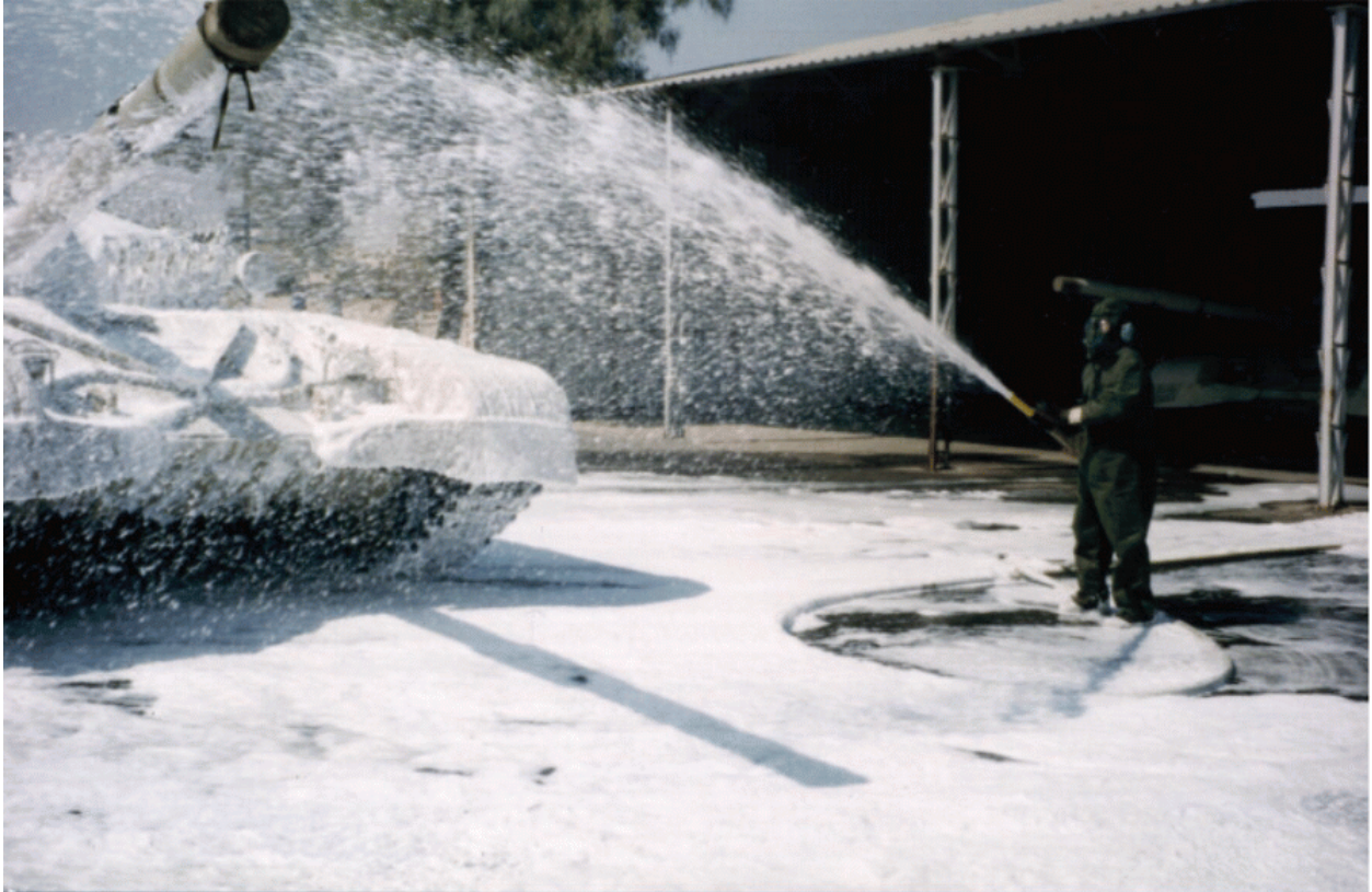
Figure 4.2-1. Demonstration of the Foam Application on a Tank Vehicle
