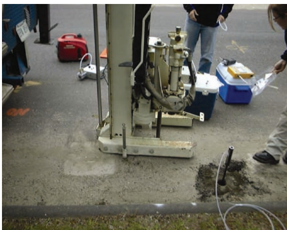
Figure 22. Proximity of dedicated vapor probe (metal cover surrounded by white concrete at base of Geoprobe unit), PRT, and GVP sampling systems.
