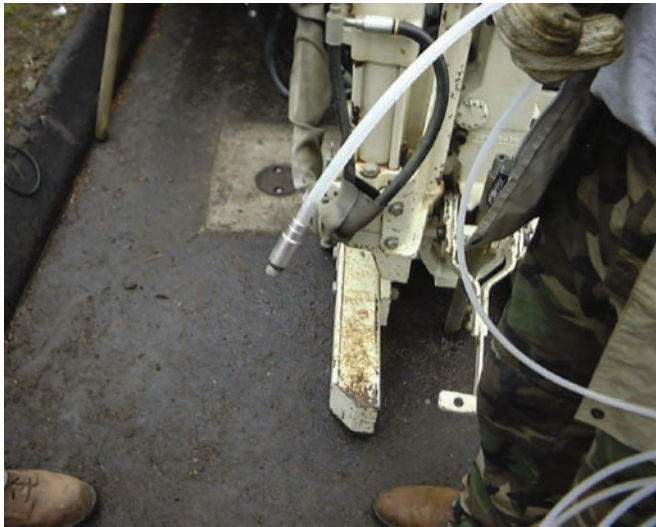
Figure 14. Photograph of a PRT adapter with an O-ring and associated Teflon® tubing.
