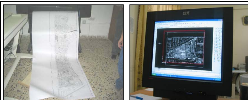
Scans of old cloth and paper maps produce a printed image map (left) and an electronic base map (right).
