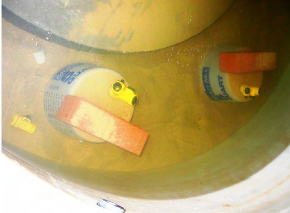
Figure 12. Paint-bucket seepage cylinders (20.25-cm-diameter) installed inside tank 2. Bricks resting on top of bucket are to counter buoyancy of the plastic. A silicone stopper and a hardware fitting are visible on the sand bed of the seepage tank. A large-diameter metal seepage cylinder is visible at the top of the photograph.
