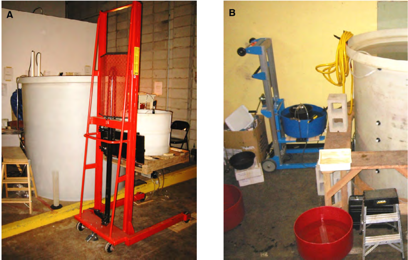
Figure 7. (A) Pneumatic foot-pump-operated fork lift used to adjust reservoir for tank 1. (B) Hand-crank fork lift used to adjust reservoir for tank 2.
