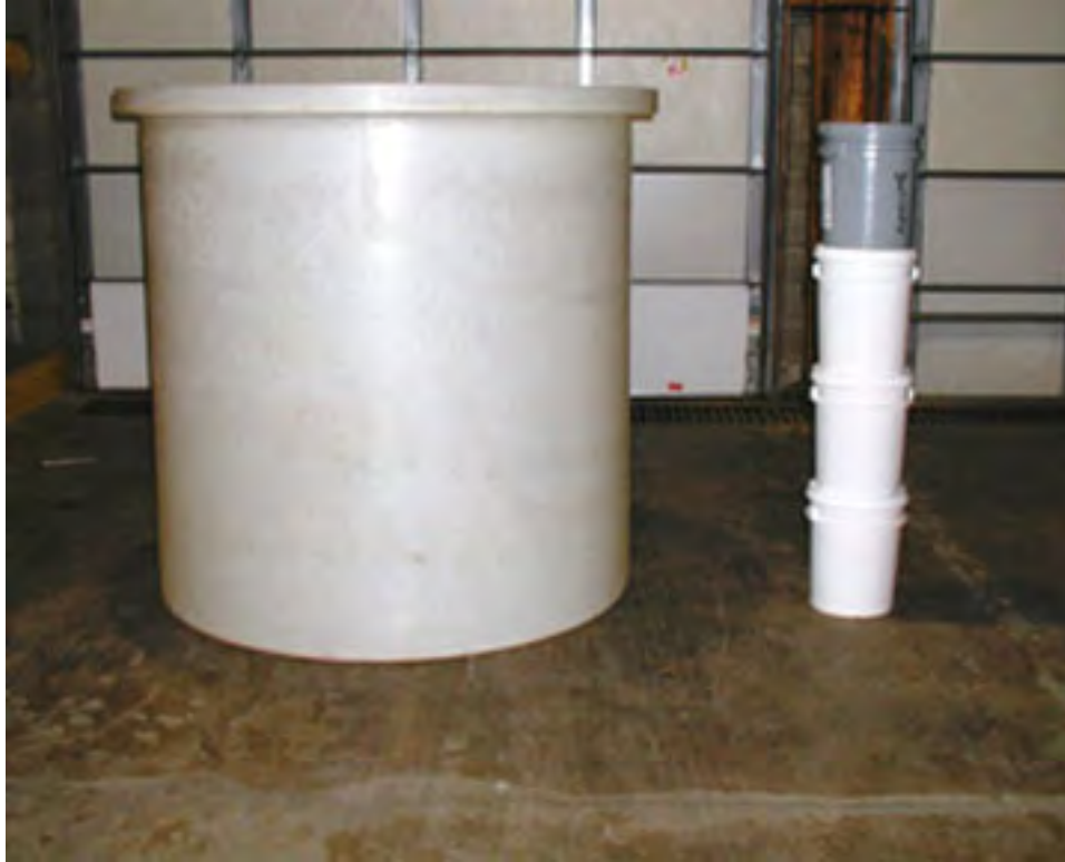
Figure 3. Plastic tank used as the flux chamber. Drywall buckets (19-liter (5-gallon)) shown for scale.
