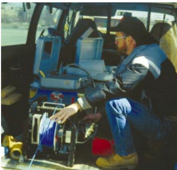
Figure 1. A PC-based geophysical logger with portable drawworks and plastic-coated logging cable in use at a contaminated ground-water site.
