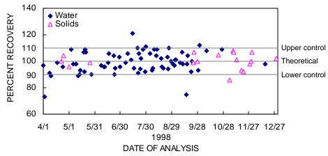
Figure 1. Percent recoveries for analyses of total mercury.
