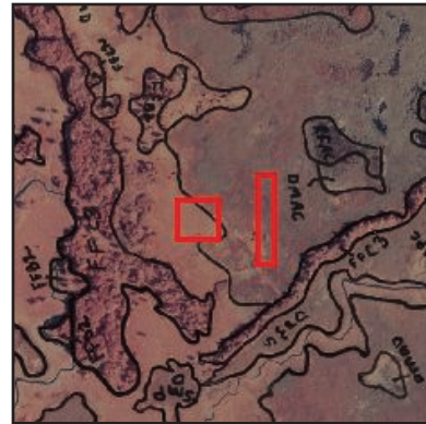
Figure 1-5. The red boxes depict two different shapes of the minimum mapping unit (1 ha or 2.5 acres) used when photointerpreting 1:24,000-scale photography.
