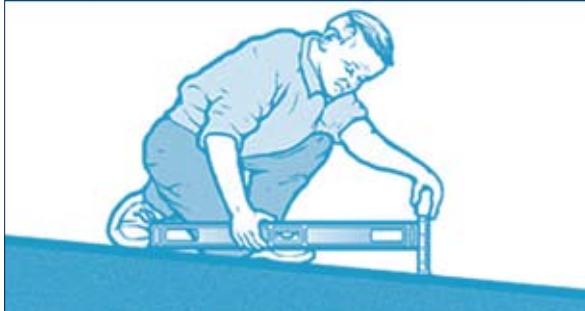
Image 9.3: Measuring slope using a 24-inch level and tape measure.
