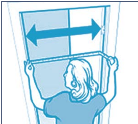
Image 9.5: Measuring the clear opening from the face of the doorstop on the frame to the face of the open door.”
