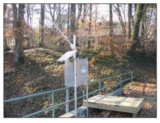
Sixty-two of the 130 sites monitored for water quality in Georgia are equipped with streamflow and water-quality instruments that collect and transmit data via a satellite linkup. These data are updated several times each day and displayed on a USGS Web site at <a href="http://ga.water.usgs.gov/">http://ga.water.usgs.gov/</a> Photograph by Andrew C. Hickey, USGS.
