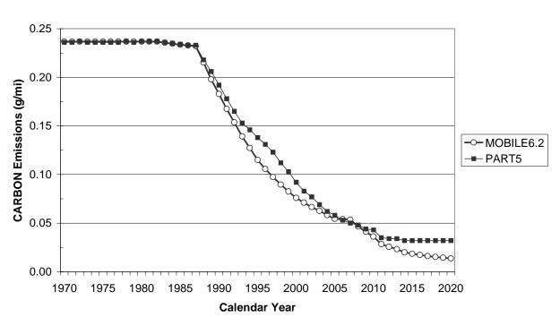
MOBILE6.1 and PART5 GASPM from Heavy-Duty Gasoline Vehicles
