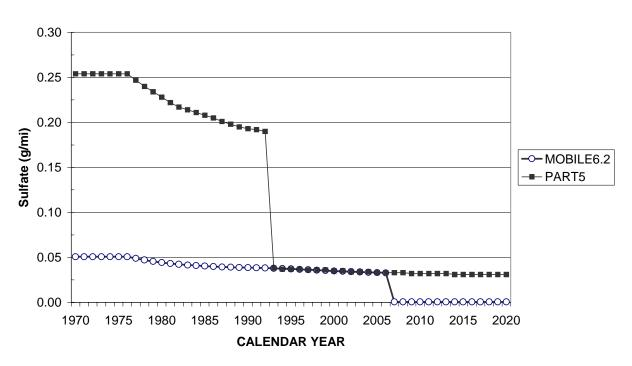
MOBILE6.1 and PART5 SULFATE Emissions for HHDDVs
