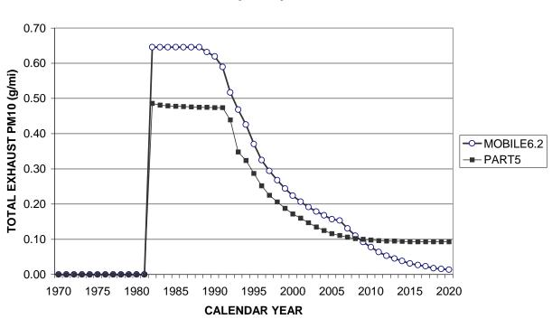
MOBILE6.1 and PART5 Total Exhaust PM10 Emissions from 2B Heavy-Duty Diesel Vehicles
