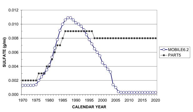
Comparison of MOBILE6.1 and PART5 SULFATE Emissions for LDGVs
