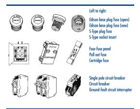
If the demand for electrical current exceeds the safety level, a fuse opens once and must be replaced to reconnect the circuit. A circuit breaker "trips" its switch to open the circuit, and the circuit is reconnected by closing the switch manually.
