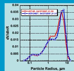
Processing with Aeronet retrieval code yields near match with co-located Cimel sun photometer.
