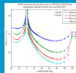
4-STAR diffuse radiance calibration at NASA ARC agrees well with NASA GSFC Cimel calibration.
