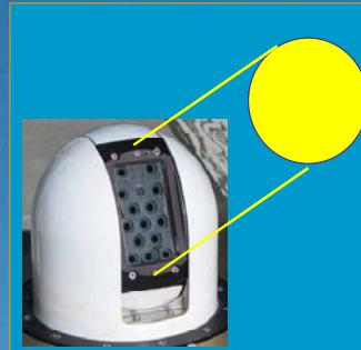
**AATS-14 like retrievals of column amount and profiles of aerosol and gaseous atmospheric components.**
