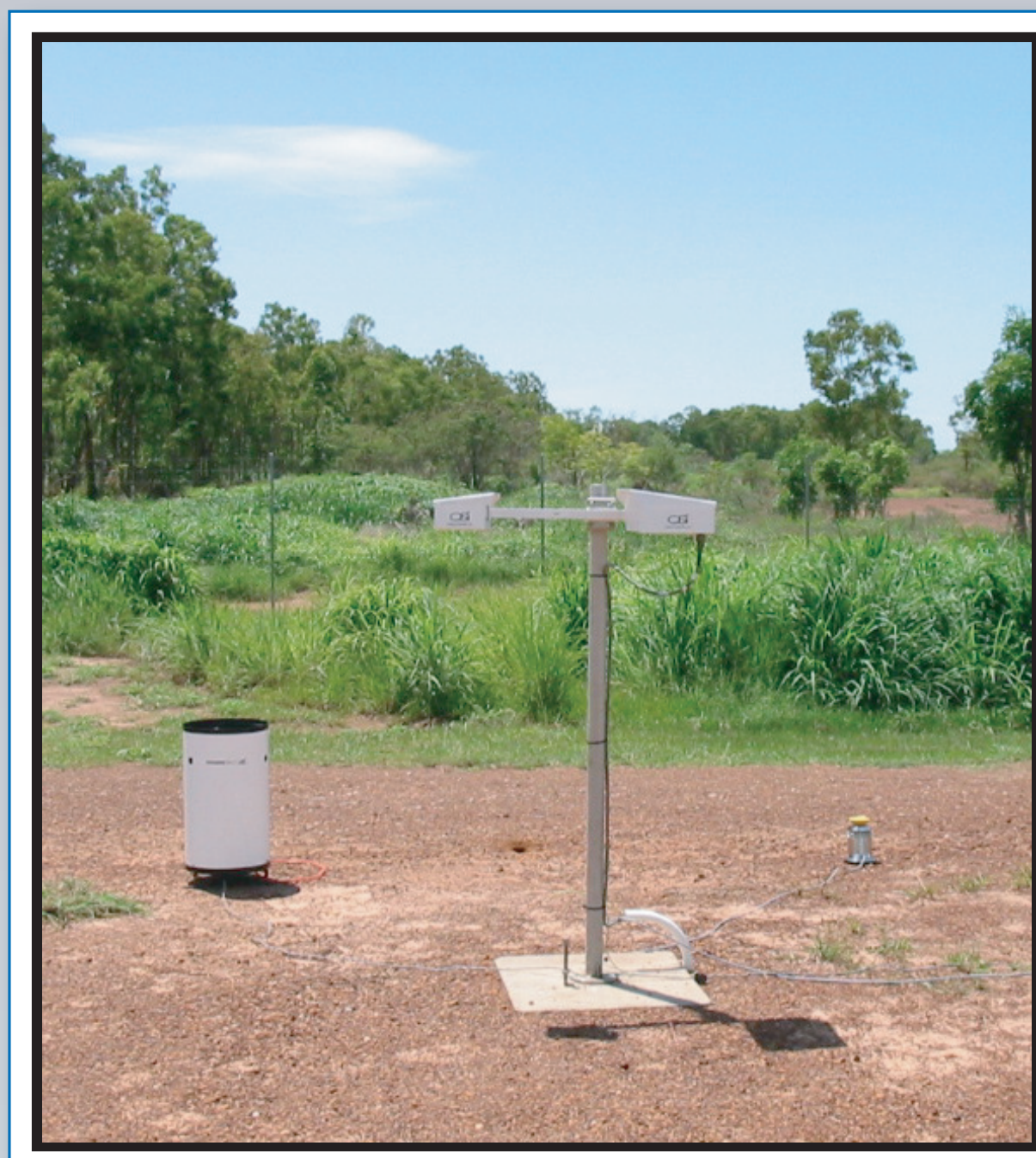
Tipping Bucket Rain Gauge (left) Optical Rain Gauge (center) Disdrometer (right) (not used in this study)
