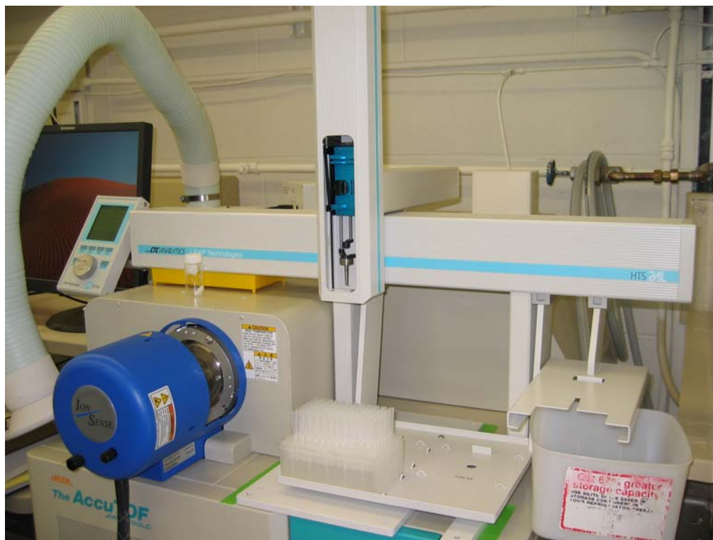
Figure 1-3. The DART-TOF system with LEAP autosampler as installed at RTI International.
