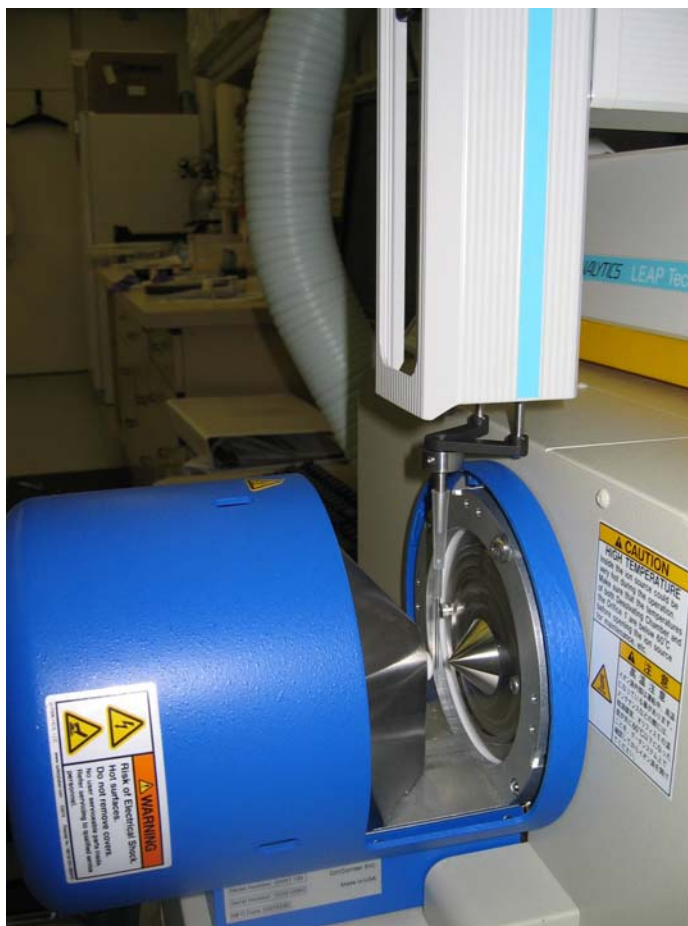
Figure 2-2. Sample introduction into the DART-TOF ion source.
