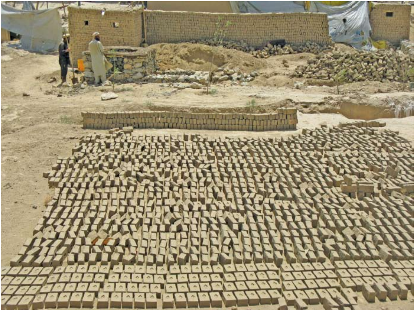
Mud bricks, constructed through a program similar to OFDA-funded livelihoods programs, dry in the sun in Afghanistan (Photo by Yoni Bock, USAID).
