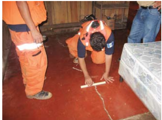
Guatemalan disaster personnel measure a crack in the floor of a house affected by landslides (Photo by Ricardo Berganza, USAID).
