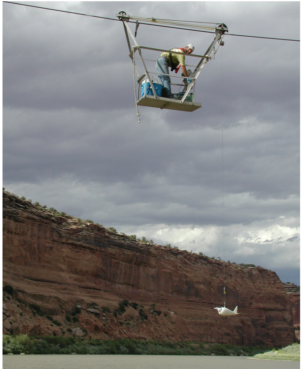
A U.S. Geological Survey scientist collects a sample from the Colorado River for analysis of dissolved solids and other water-quality constituents (USGS photograph by Nancy Bauch).
