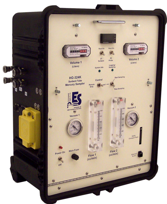
Figure 2-1. HG-324K Sorbent Tube Mercury Sampling System
