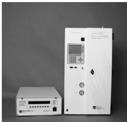
Figure 2-1. Rupprecht & Patashnick, Co. Series 8400S Particulate Sulfate Monitor
