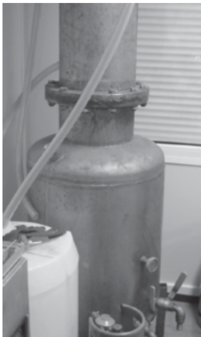
Custom made pressure reaction vessel. Synthetic Drugs Unit Helmond, Holland 6-7-2004.
