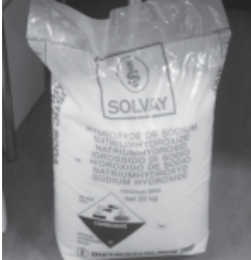
Sodium hydroxide – reagent used in the production of ATS. Corrosive to human tissue and can cause eye and tissue burns, and nerve damage.
