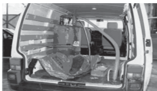
With the use of a compressor, connected to the car cigarette lighter, chemical waste from ATS production was dumped from this vehicle via a PVC pipe, along a road in the Netherlands. Source Synthetic Drugs Unit, Helmond, Holland.
