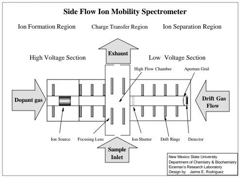
Figure 2. Schematic representation of the IMS used in these studies, which was designed and built at New Mexico State University
