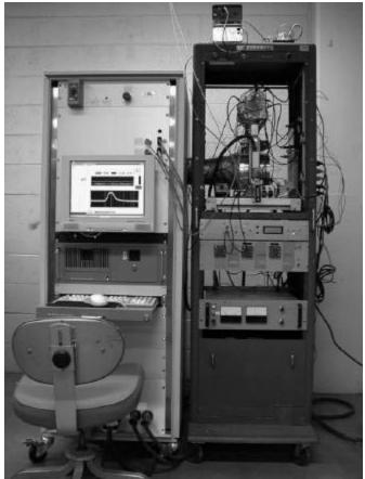
Figure 4b. Power racks containing the IMS, preconcentrator, and system controls
