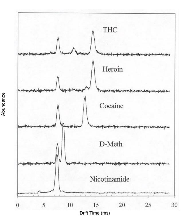
Figure 7. IMS spectra for different drugs with the use of nicotinamide dopant. The quantity of drug injected is 1 **mg** in all cases except for THC where 100 ng was used
