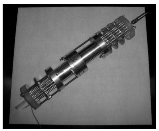
Figure 3. Photo of the IMS. The ion formation region is at the lower left
