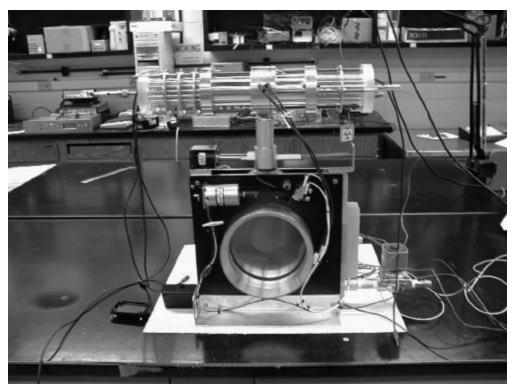
Figure 4a. The IMS mounted on top of the Sandia preconcentrator
