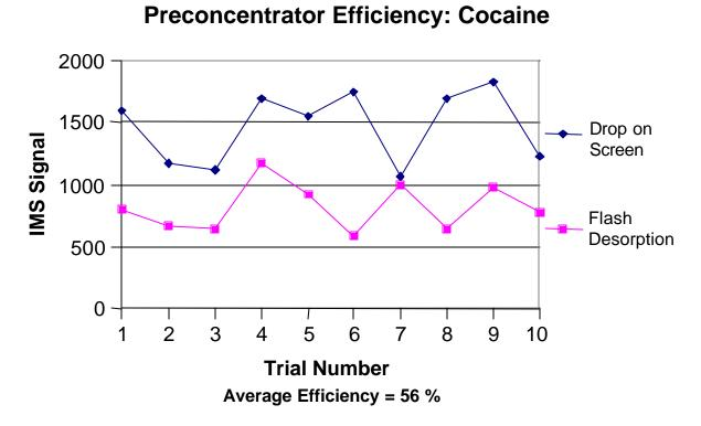
Figure 9. Set of 10 measurements used to estimate preconcentrator collection efficiency for cocaine
