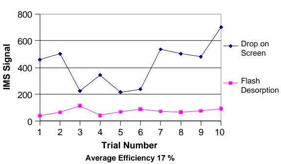
Figure 10. Set of 10 measurements used to estimate preconcentrator collection efficiency for heroin
