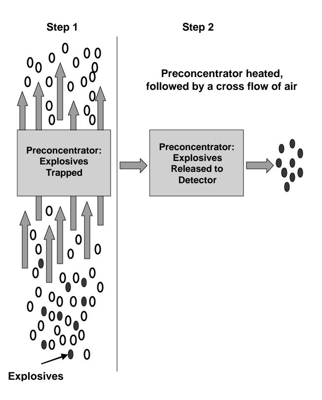
Figure 5. Schematic representation of the trapping of analyte molecules in the preconcentrator, with subsequent delivery to the detector
