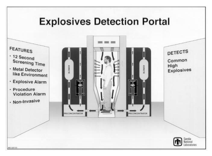
Figure 1. Schematic representation of the explosives detection portal developed at Sandia National Laboratories
