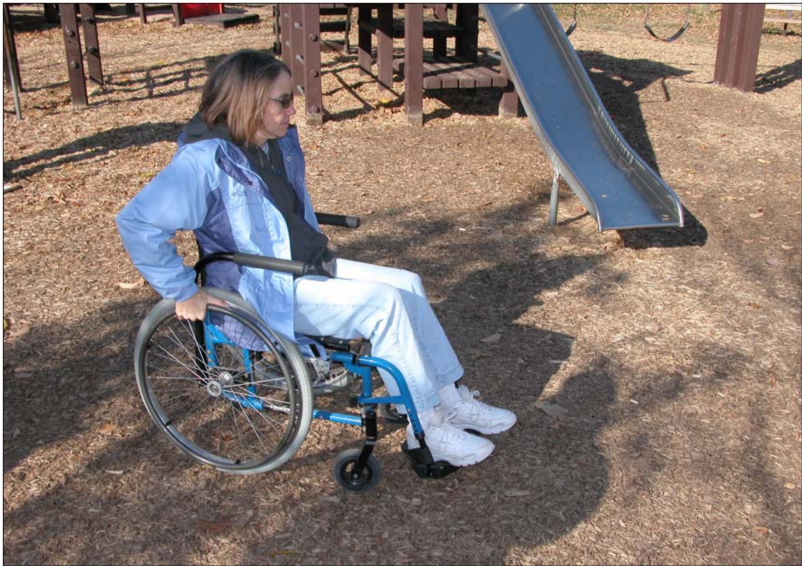
Figure 8—Completed playground looking north: left, Vitri-Turf SEWF; right, Soil-Sement SEWF; top, EWF. Line of demarcation is below wheelchair footrest.
