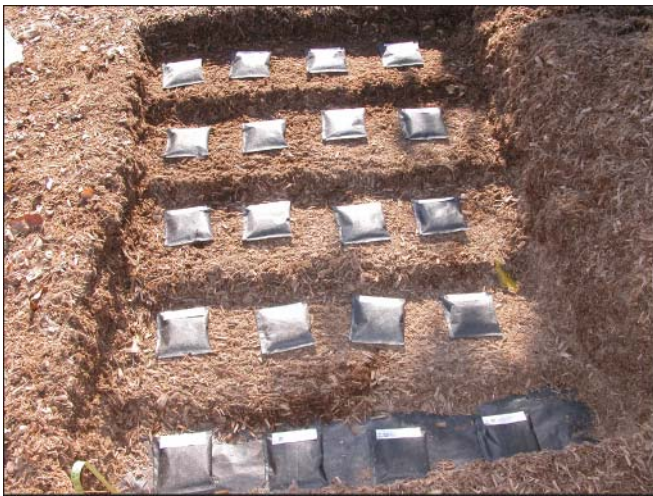
Figure 11—Biodeterioration samples on EWF surface.
