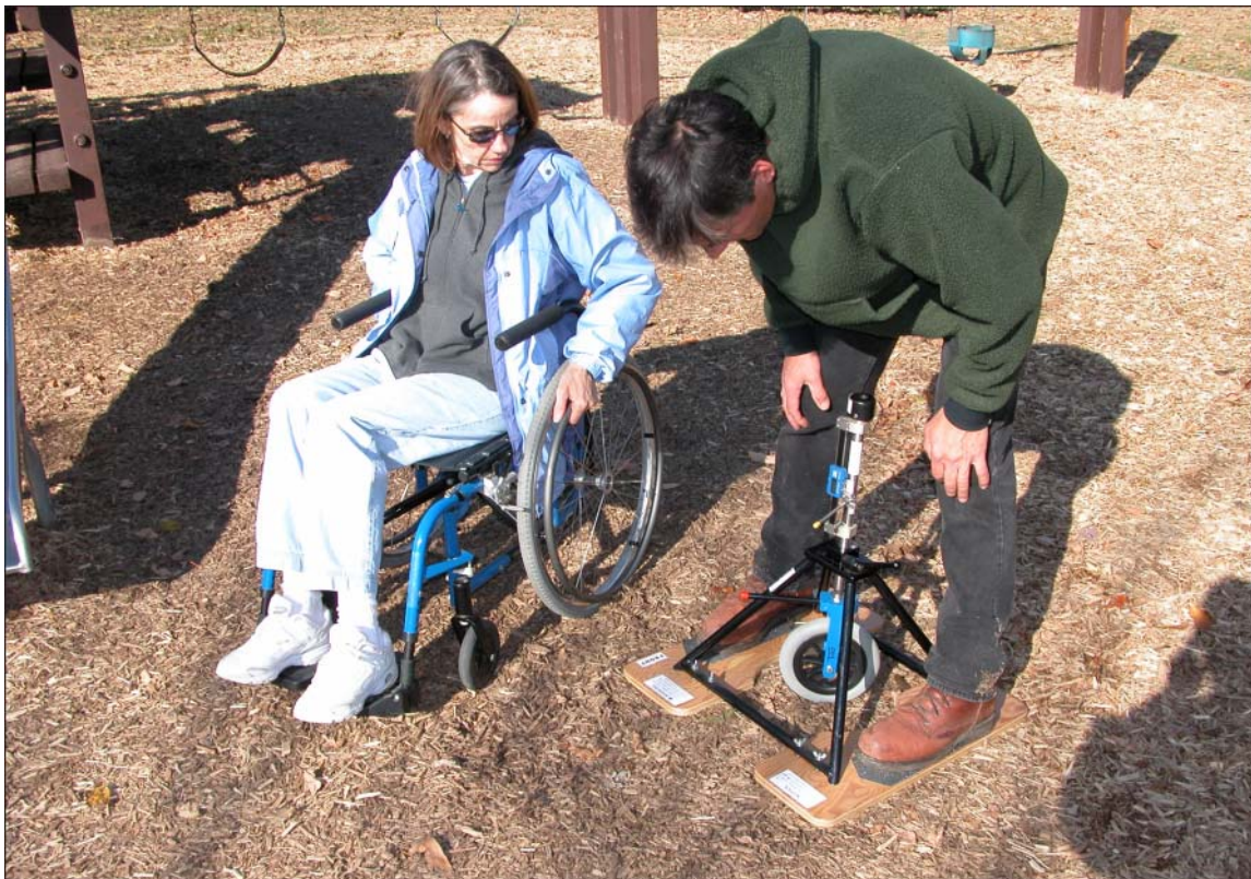
Figure 9—Measurement of accessibility with rotational penetrometer.
