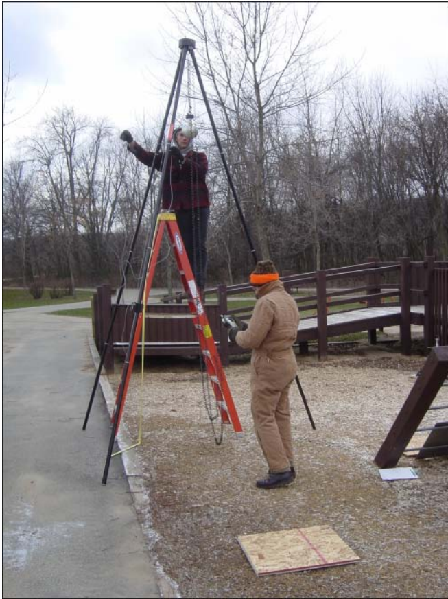
Figure 10—Impact test setup for drop height of 3.05 m (10 ft).
