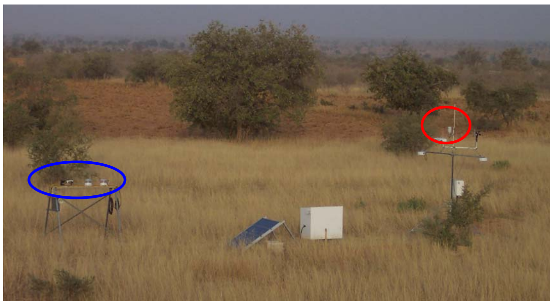
Figure 25. Picture of the S1 site radiometer and met instruments. Red circle is the ambient air temperature and moisture sun-shielded enclosure, blue circle is the downwelling radiometers.
