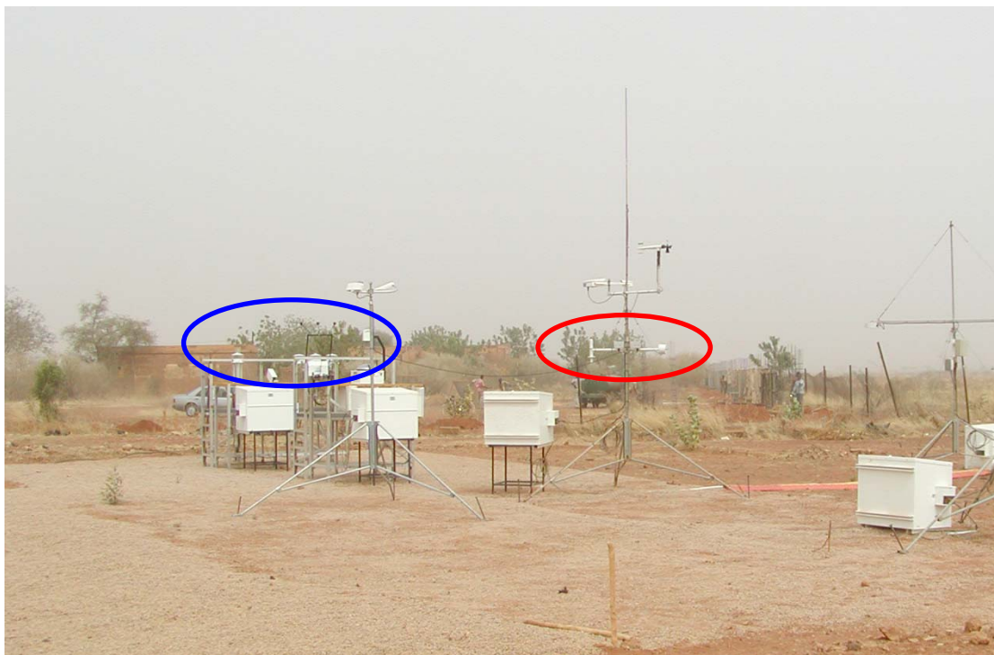
Figure 24. Picture of the N1 site radiometer and met instruments. Red circle is the ambient air temperature and moisture aspirated enclosure, blue circle is the downwelling radiometers.
