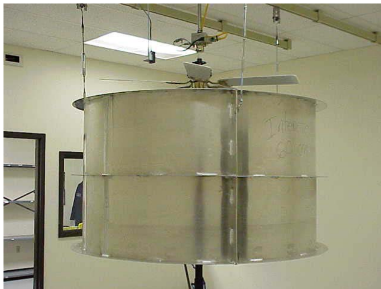
Figure 4.4 – Ceiling Fan Testing Set-Up
