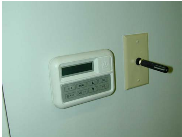
Figure 4.1 – Temperature and Humidity Sensors in Testing Room
