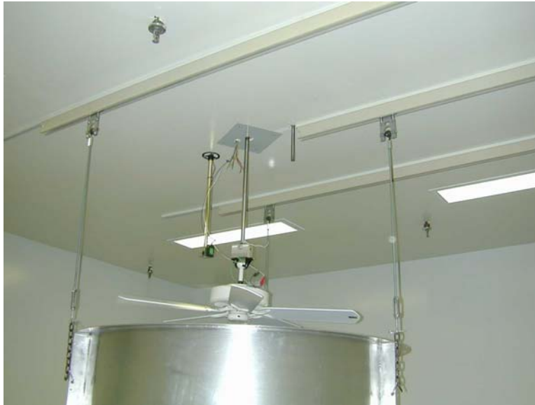
Figure 3.3 – Test Cylinder and Rail Track Support
