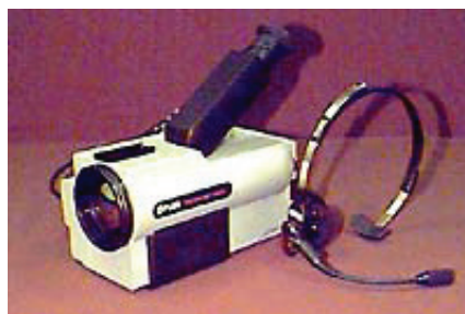
The FLIR ThermaCAM P20 infrared camera is one of nine types of infrared cameras Western customers can borrow from the Equipment Loan Program.
