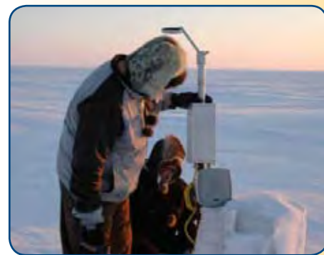
ACRF operations staff Walter Brower (standing) and Jimmy Ivanoff (kneeling) reinstall the total precipitation sensor near the Great White instrument shelter in Barrow.
