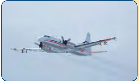
The Convair takes off on one of its 16 flight days from Fairbanks to Barrow, Alaska, during the month-long ISDAC field campaign. Both wings were heavily instrumented with cloud and aerosol probes.
