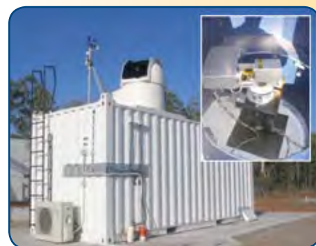
A camera, weather station, and sun tracker with a protective dome are located on the roof of the fully automated FTS mobile laboratory. Inside the shelter, the spectrometer receives the reflected solar beam from the sun tracker (inset), while the main computer system operates all the instruments and acquires the data.
