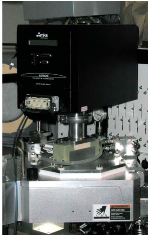
Figure 7-6. Astron Remote Plasma Source (for NF 3 CVD chamber cleaning), an important technology for reducing PFC emissions from semiconductor manufacturing.
