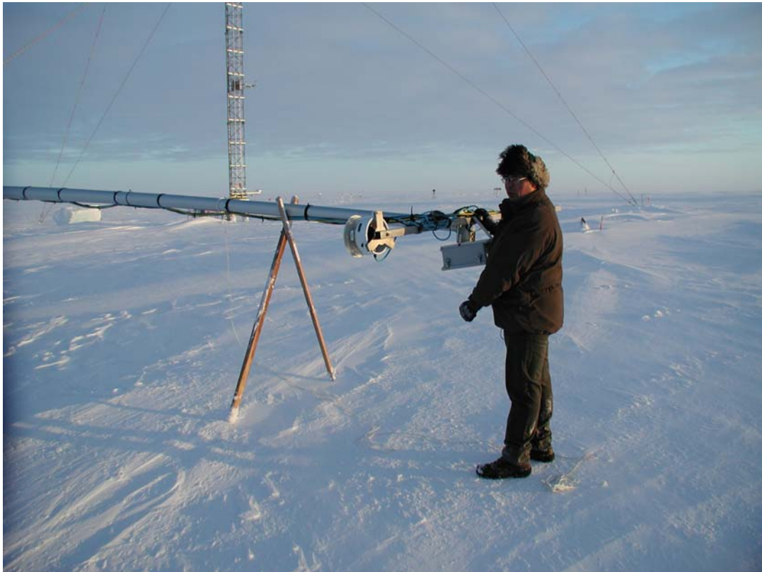
Figure 4 The tower in the lowered position supported by the wooden frame. A counterweight is necessary to hold the tower in the horizontal position.
