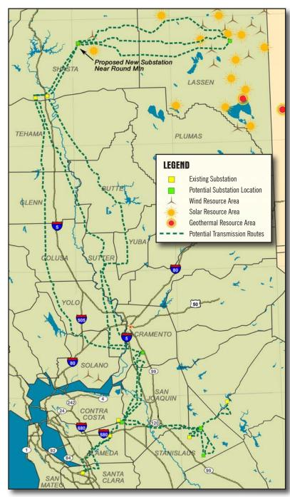
Preliminary proposed transmission routes shown here represent <u>multiple</u> alternatives that will be evaluated during the environmental review (CEQA/NEPA) process. For each segment of the program, a <u>single</u> route will connect existing and proposed substations, except east of the Proposed New Substation Near Round Mtn., where two 500kV lines will be sited.
