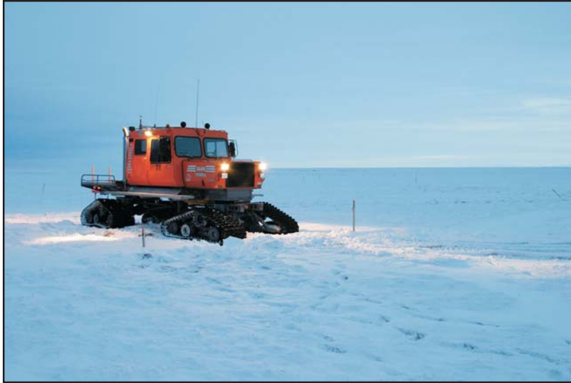
Tracked vehicle of the type used for many years for tundra access in winter. Vehicles with very wide tires called rollagons are also used for this purpose.
