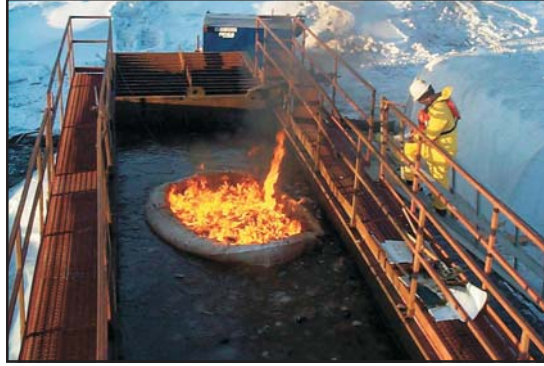
Test burn with crude oil on frazil ice.
