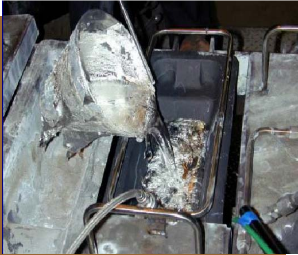
Figure 1. Molten Mg with SF 6 cover gas.
