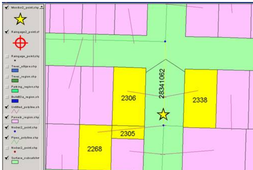
Figure 14-10. Close-up of parcels draining to pipe 62. Monitor (star) is actually downstream of entry of DCIA drainage from subcatchments 2268 and 2305. Likewise, the surface area of these two subcatchments drains north (up in figure) to enter pipe 62 above its drainage divide.
