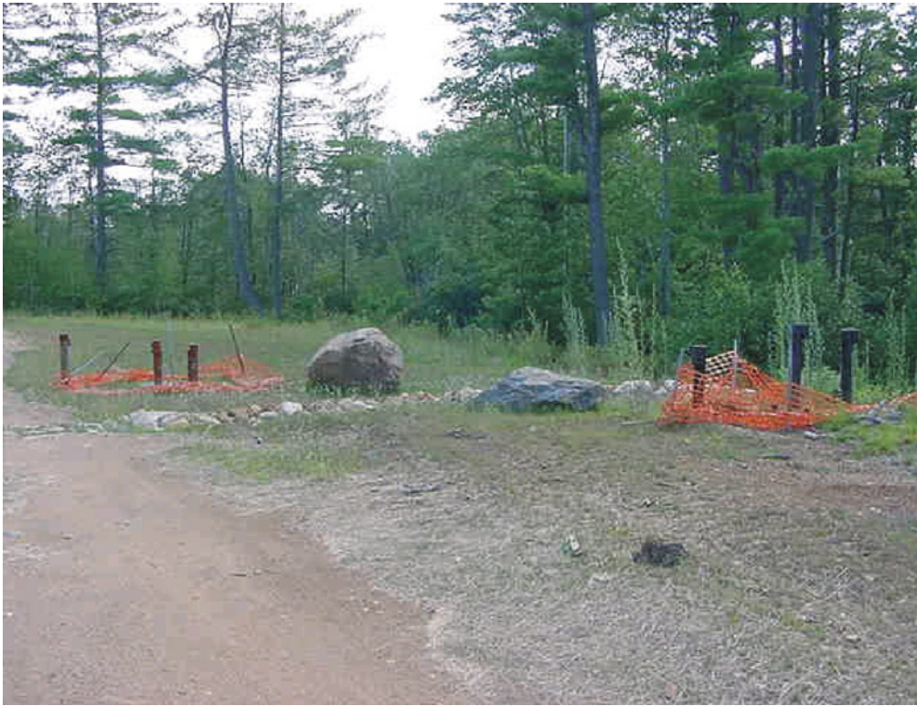
Monitoring Wells on the Landfill's West Side
