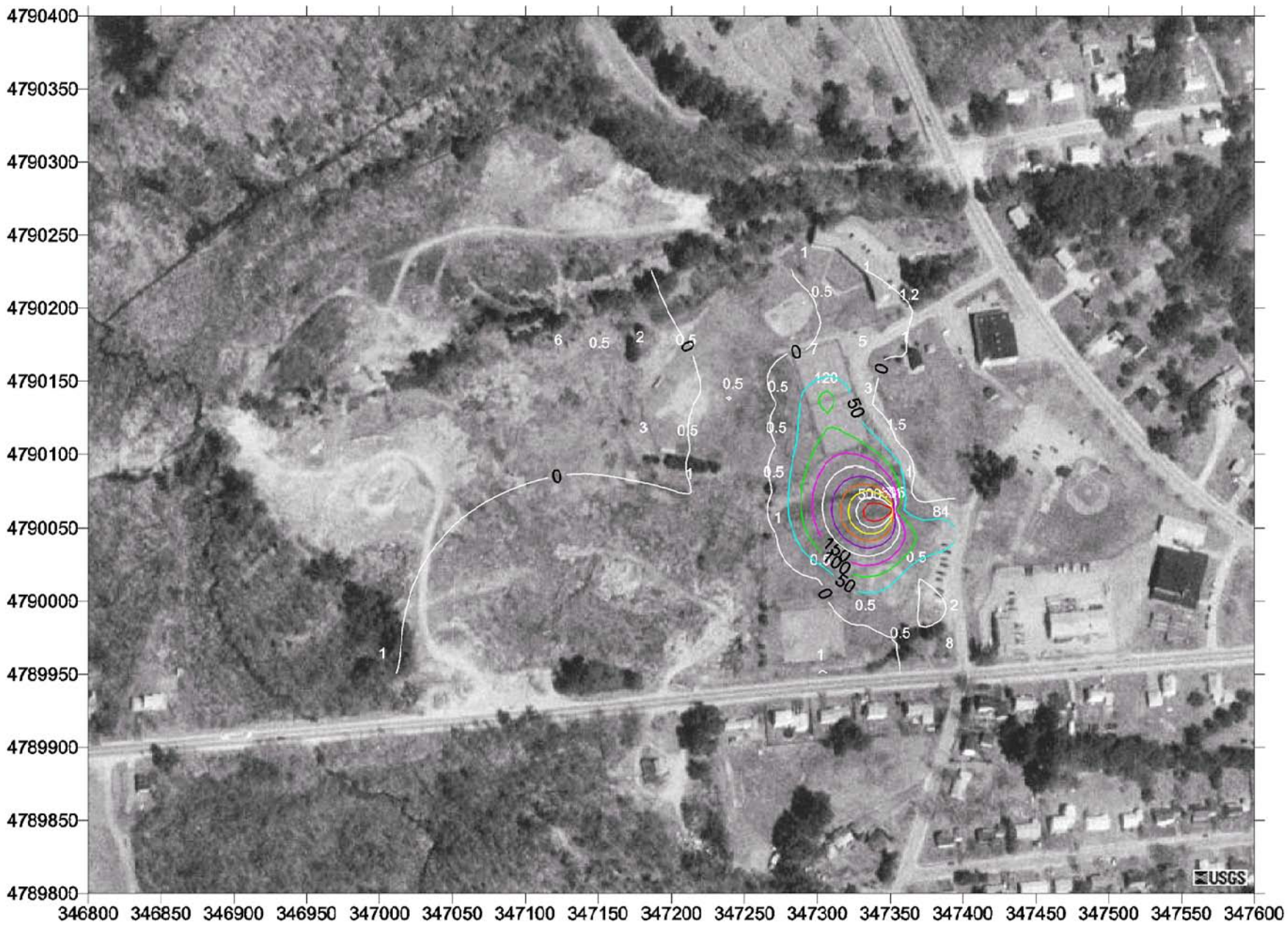
Figure 4. Measured Screening Results for Methane (ppm)
