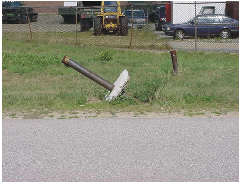
Damaged Monitoring Well
