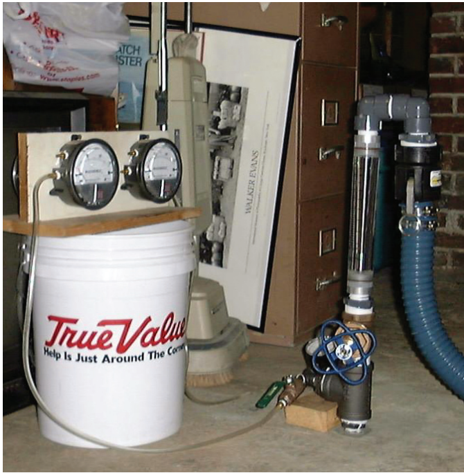
Figure 23. Variable-area flowmeter used for air permeability testing.
