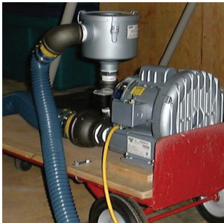
Figure 22. Regenerative blower used for air permeability testing.
