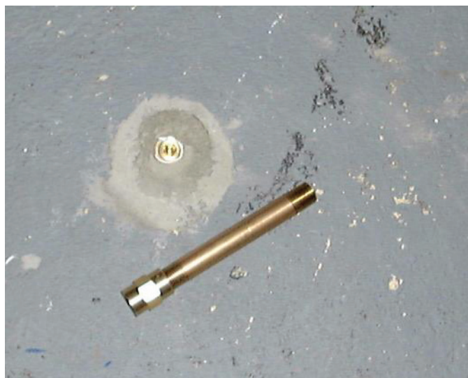
Figure 11. Brass materials used for sub-slab probe construction in homes near the Raymark facility.
