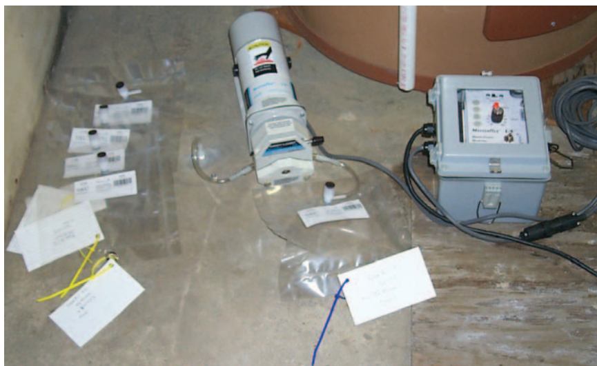
Figure 19. Sample train for sub-slab air collection using one-liter Tedlar bags.
