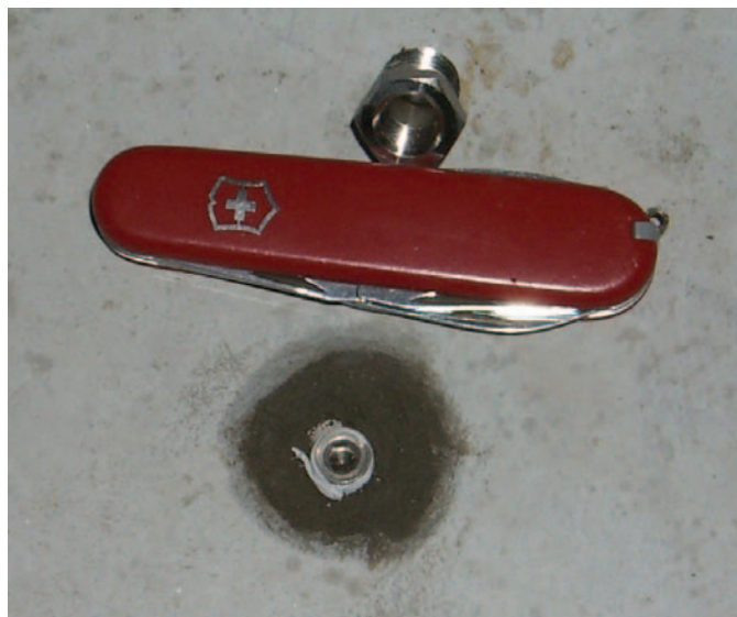
Figure 12. Hex bushing used for probe construction when a concrete slab was less than 2.5 cm thick.
