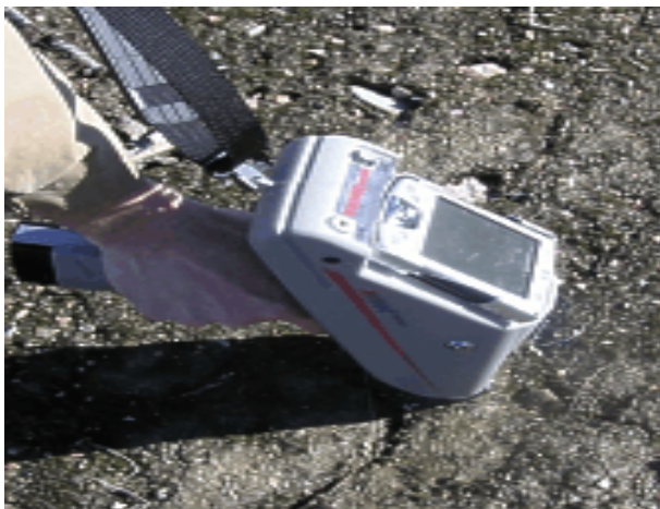
Figure 6-1. Oxford X-Met 3000TX set up for portable in situ analysis.
