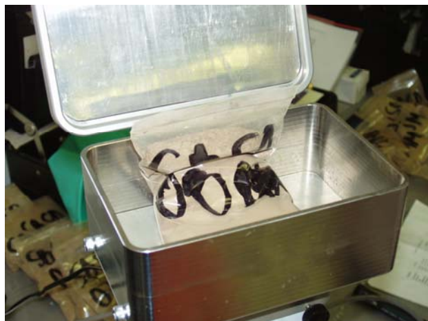
Figure 6-3. Oxford X-Met 3000TX sample container with sample.
