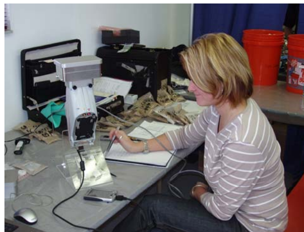
Figure 6-2. Oxford X-Met 3000TX set up for bench-top analysis.
