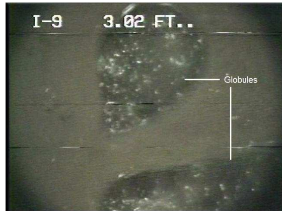
Figure 2-4. Globules of PCE in the near-surface fill material (from Video-CPT).
