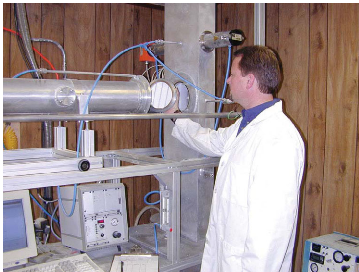
Installing a fabric swatch in the test apparatus
