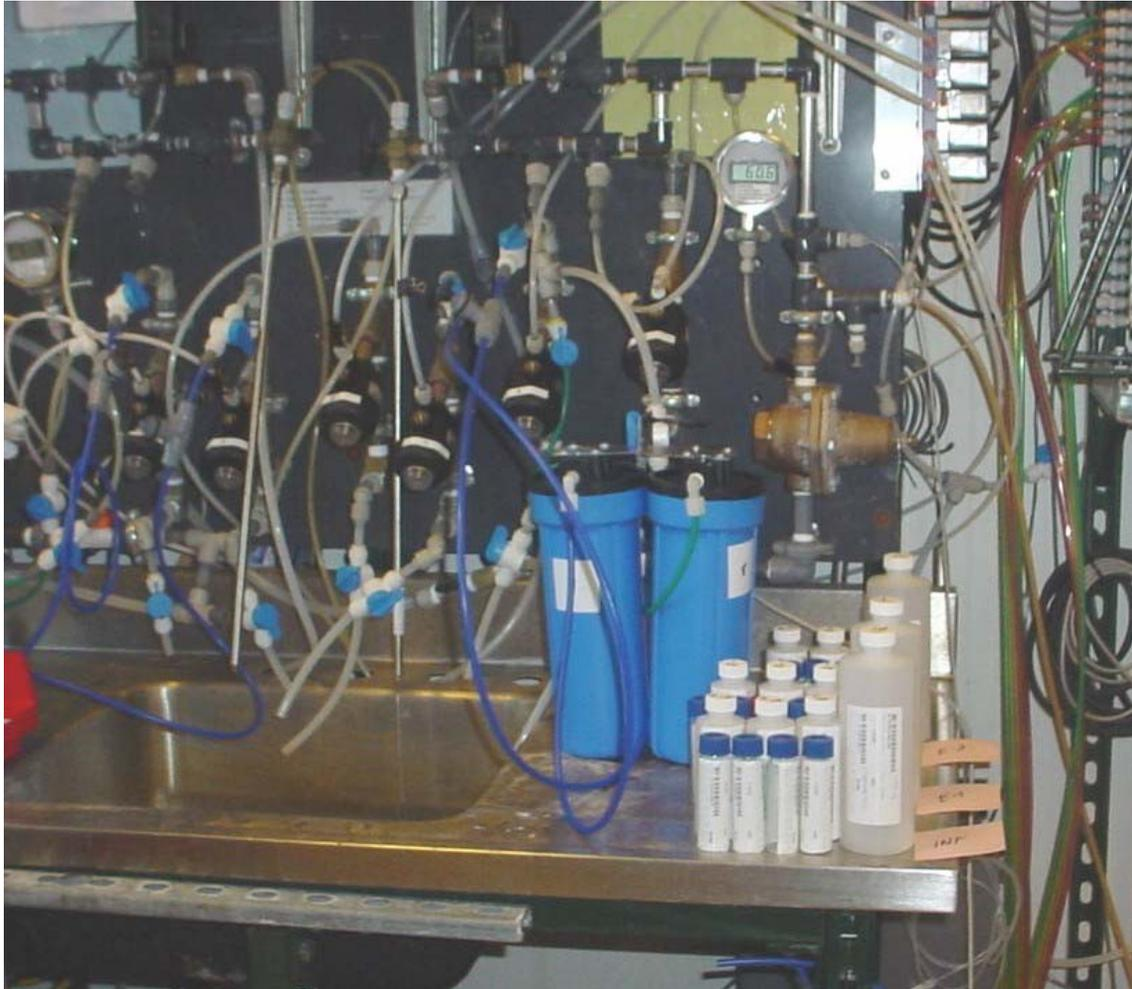
**Figure 3-2. Post-Membrane Carbon Filters Installed at Test Station**
