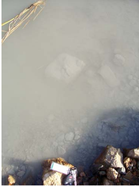
Figure 3-7. Photograph showing evidence of excess sulfur in the shallow pit water after hydrogen peroxide addition.
