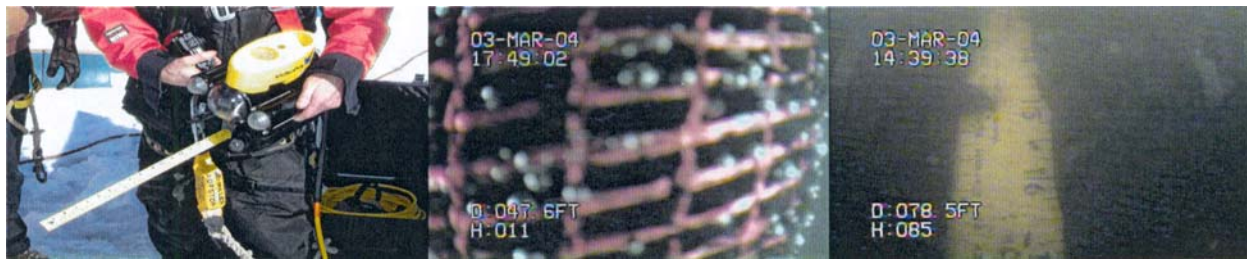
Figure 3-2. Camera used for video camera observations (left), gas bubbles within suspended bags of chips (center), and sludge at bottom of pit (right).
