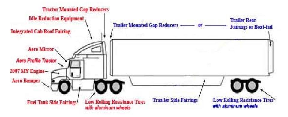
Potential fuel savings – 10% - 20% (on-highway operation) compared to a truck without these features
