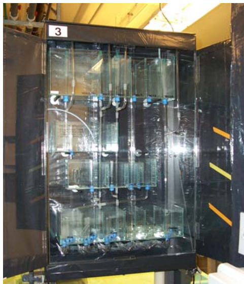
Figure 2.1. Continuous flow proportional diluter system
