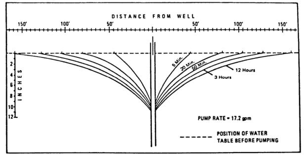
Figure 10-12: Diagrammatic Illustration of Development of a Cone of Depression Based on an Actual Aquifer Test
