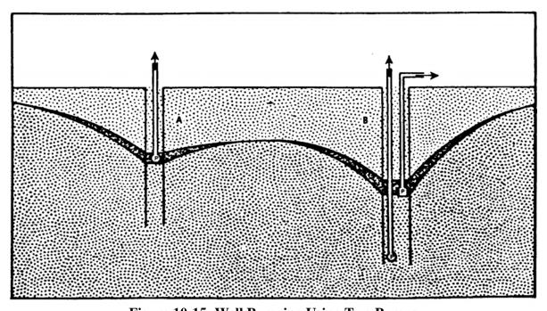
Figure 10-15: Well Pumping Using Two Pumps Well A is maintaining depression and recovering oil in a single operation by drawing the fluid surface down to the pump level. Well B is maintaining depression by pumping clean water from below the water table. Floating oil is recovered by a suction pump at the fluid surface.
