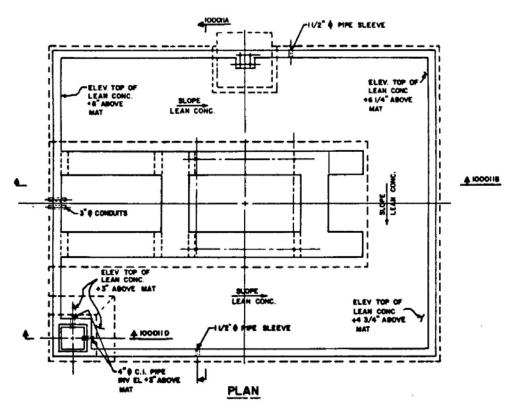
Figure 6-13: Plan View of Equipment Pit
