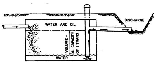
Figure 6-10: Typical Construction of Oil Separator Tank
