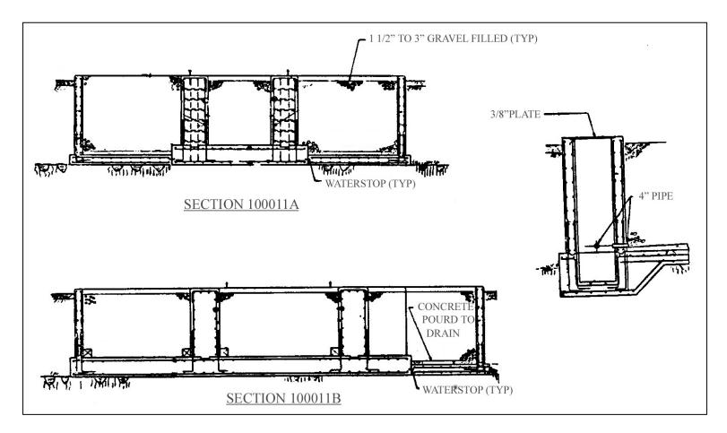
**Figure 6-14: Details of Equipment Pit**
