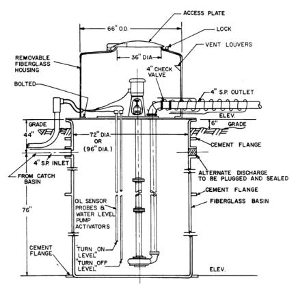
**Figure 6-19: Above-Grade Sump Pump Discharge**
