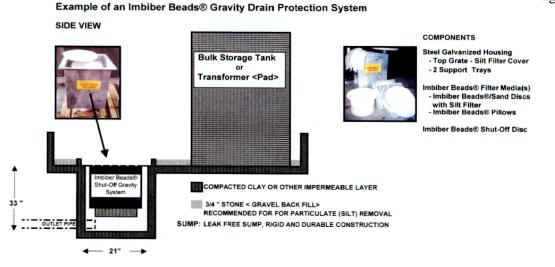
Figure 6-8: Example of an Imbiber Beads<sup>®</sup> Gravity Drain Protection System
