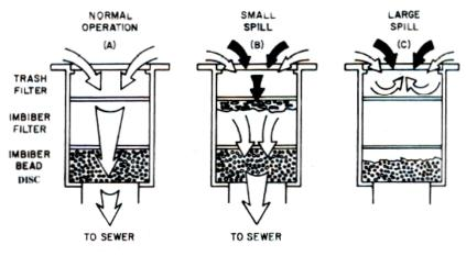
**Figure 6-7: Imbiber Beads**<sup>®</sup> **Gravity-Flow Drain Protection System–Operational Process**
