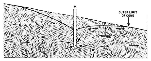
Figure 10-14: Drawdown Configuration of Well Pumping From Inclined Water Fluid at the surface of the water table between the divide and outer limit of cone will not be trapped, but will move down gradient with the water.
