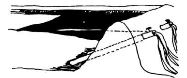
Figure 7-14: Earthen Dam, Cross Section Pipes installed on an incline to control water depth. The top of the incline determines the height of the retained water and oil.
