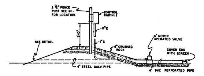
Figure 6-21: Motor-Operated Gate Valve
