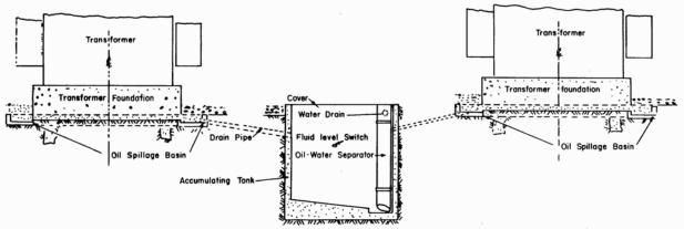
Figure 6-11: Transformer--Accumulating Tank Combination
