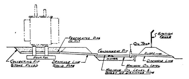
Figure 6-3: Cross Section of Oil Drainage System
