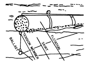
Figure 7-1: Components of a Boom
