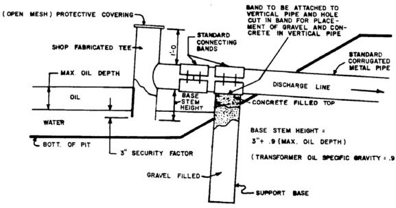
Figure 6-4: Oil Trap or Skimming Unit
