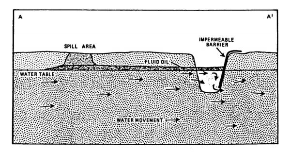
CROSS SECTION Figure 10-8: Oil Moving with Shallow Groundwater Intercepted by Ditch Constructed Across Migration Path
