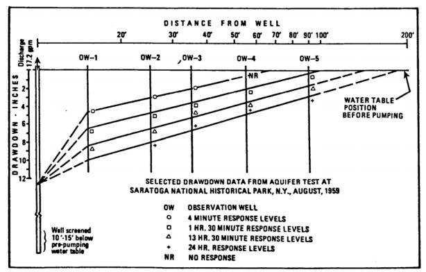
Figure 10-13: Selected Drawdown Data for an Aquifer Test
