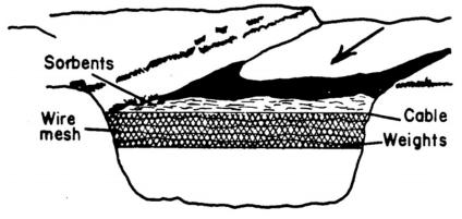
Figure 7-15 : Cross Section of a Sorbent Fence Weights on the bottom of the wire mesh keep it from planing and releasing the sorbent and oil.
