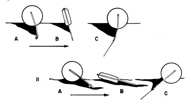
Figure 7-4: Boom "Planing" in Current I. In low current situation, oil is held by each boom type: (A) weighted flexible skirt, (B) rigid skirt, and (C) bottom tension.
