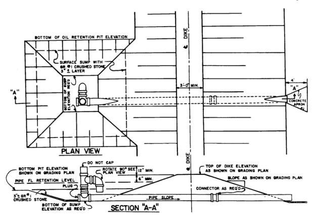
Figure 6-6: Oil Trap Construction Using Galvanized or PVC Pipe
