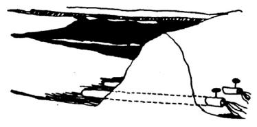
Figure 7-13: Earthen Dam, Cross Section Multiple pipes near the bottom with valves to control the flow and retained depth of the water.
