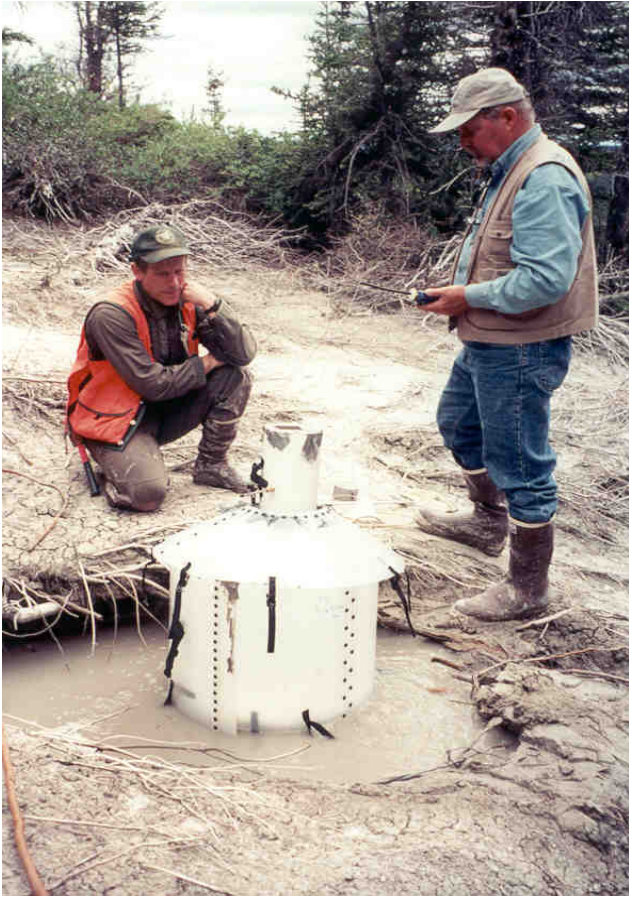
Figure 6. Equipment used to measure the rate of degassing from cold-temperature vent #6 (see figure 2 for location). Gas flowed upward through the plastic cylinder and exited through a smaller-diameter neck at the top, where its velocity and temperature were measured. The mass flow rate per unit surface area was 0.46 t/d/m 2 .
