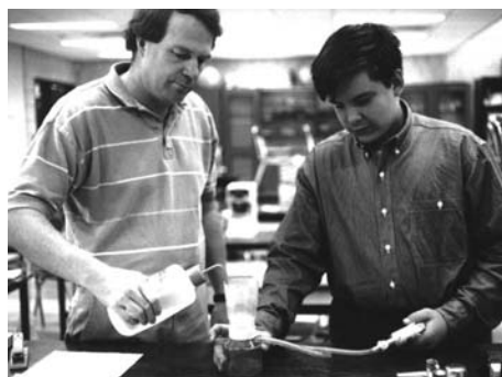
Volunteers using membrane filtration equipment. The person on the right is using a hand-operated vacuum pump to pull rinse water through the membrane filter (photo by E. Ely).
