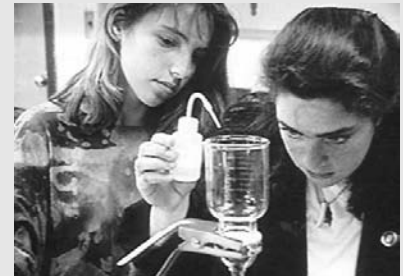
Students participating in Maine's Shore Stewards Program run estuary samples for fecal coliform bacteria using the membrane filtration method (photo by University of Maine Cooperative Extension).
