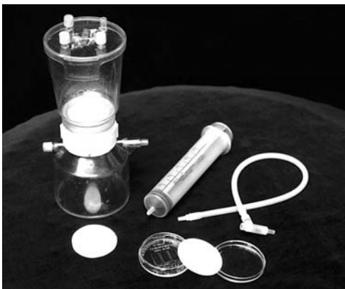
Membrane filtration equipment. Clockwise from left: membrane filtration apparatus; hand vacuum pump (syringe and tubing); petri plate with absorbent pad; membrane filter (photo by M. Redpath).
