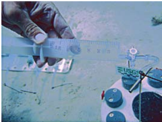
Photo 12. Water sampling syringe and mini-piezometer used for collection of reef sediment pore waters.
