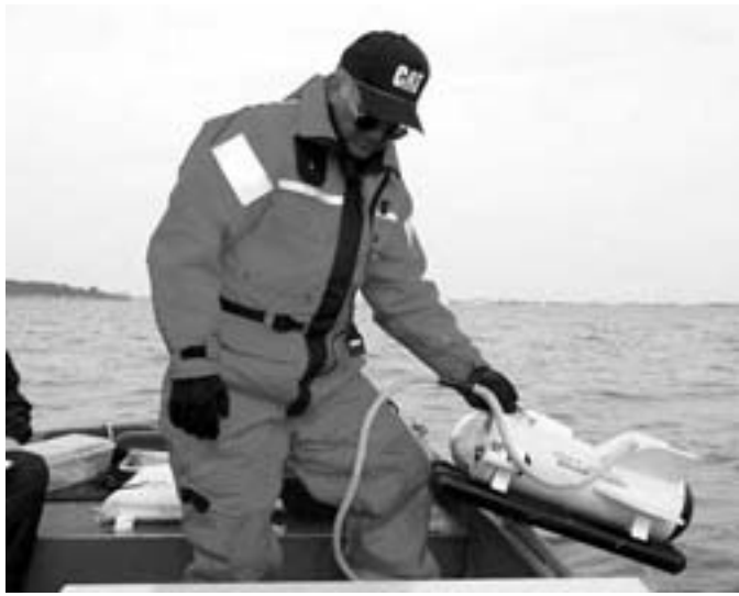
Photo 3 Towed underwater camera for field verifications.
