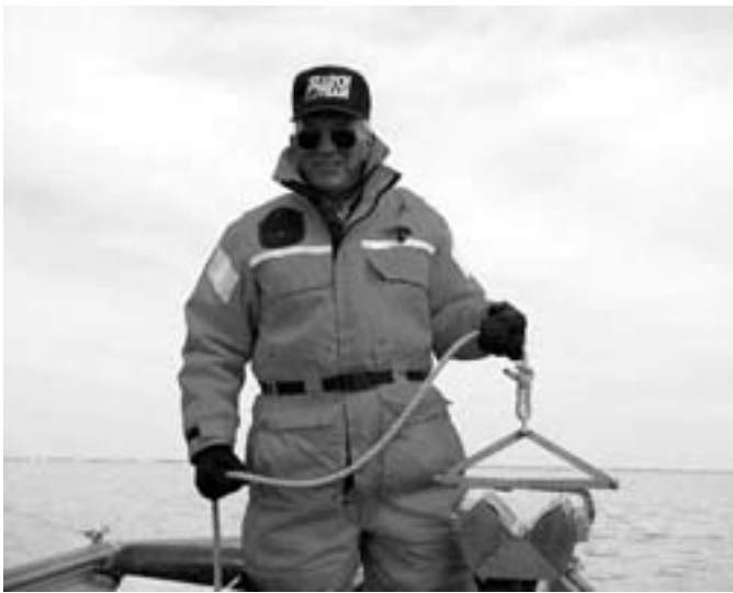
Photo 5 Petite Ponar benthic grab sampler for field verifications.
